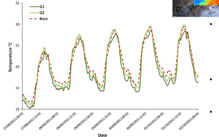
Damaged green roof performs poorly for surface temperature (Tsurf) and long recovery time
